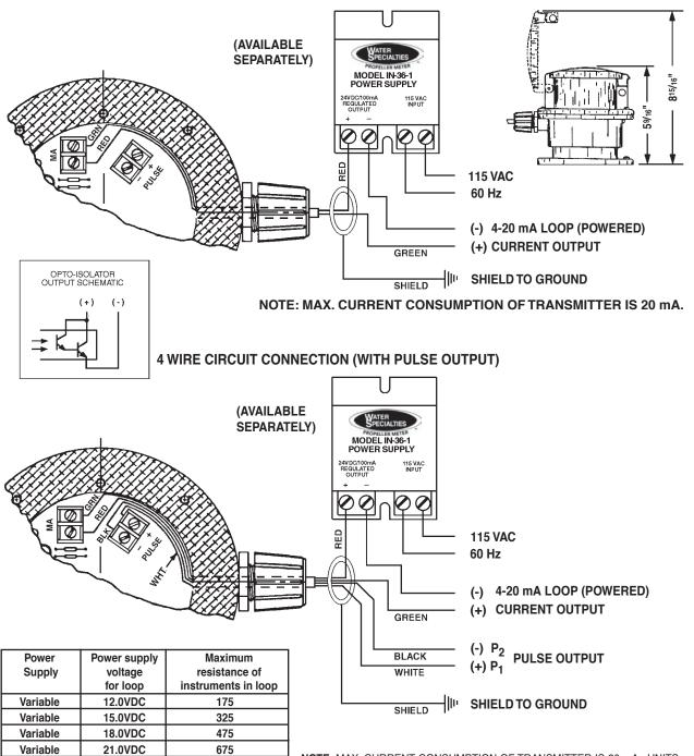
**NOTE:** MAX. CURRENT CONSUMPTION OF TRANSMITTER IS 20 mA. UNITS WHICH ARE PROVIDED WITH ONLY 2 OUTPUT WIRES MAY BE REWIRED FOR 150 PPM PULSE OUTPUT BY STRIPPING BACK THE INSULATION ON BOTH ENDS OF THE OUTPUT CABLES AND WIRING AS SHOWN ABOVE.
