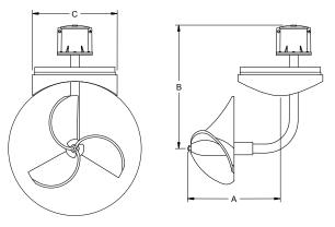
**REGISTER**: An instantaneous flowrate indicator and six-digit straight-reading totalizer are standard. The register is hermetically sealed within a die cast aluminum case. This protective housing includes a domed acrylic lens and hinged lens cover with locking hasp.
