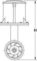
**IMPELLER**: Impellers are manufactured of high-impact plastic, retaining their shape and accuracy over the life of the meter. High temperature impeller is optional.
